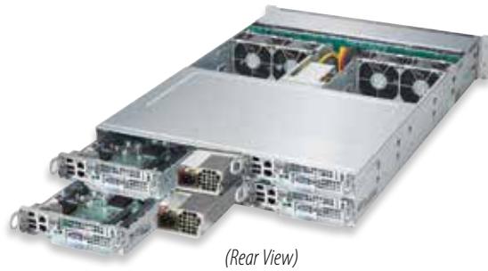
2U TwinPro™ 4 hot-swap nodes in 2U w/ 2.5" or 3.5" HDDs
