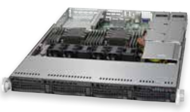
X11 WIO 1U 4x 3.5" Drive Bays Redundant Power
